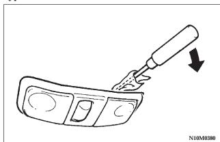
**NOTE**: Wrap a cloth around the tip of the screwdriver to avoid scratching the light assembly.
